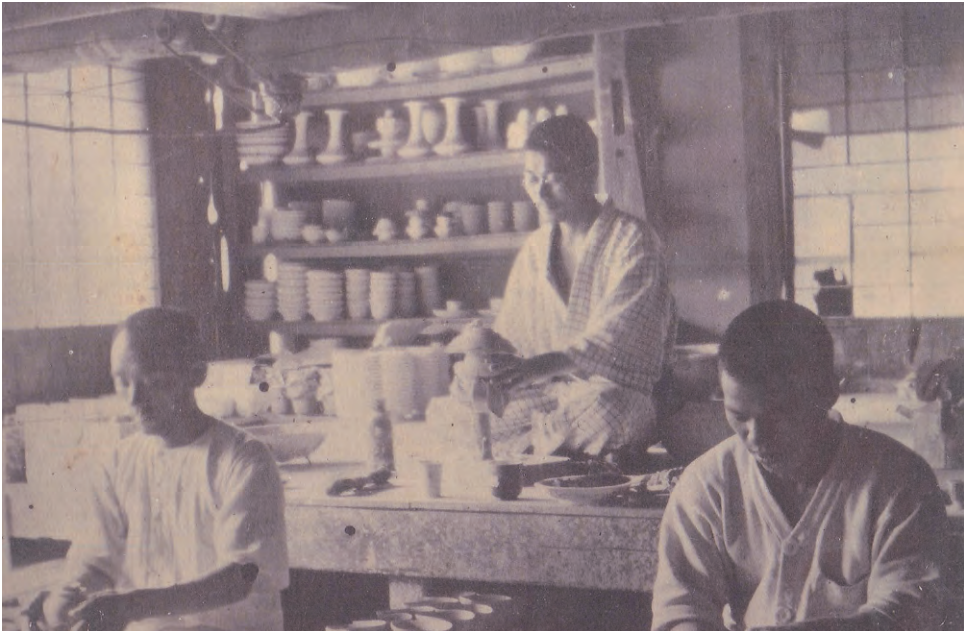
The workshop in the Meiji Era (1868-1912). Men are sitting cross-legged, throwing (front). Another is doing trimming work
